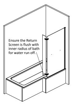
Slide the wall profile (3) onto the screen. Sit the screen onto the bath and adjust so the Return Screen butts upto the inside radius of the bath. Mark the position of the wall profile (3) with a pencil.
