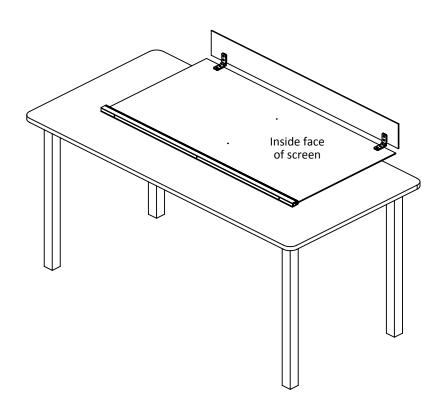
Lay front screen (1) on a flat surface to fit the return screen (2). Use the hinges provided (5). The hinge fixing screws should be to the inside face of the screen. (Do not mark the aluminium profile)
